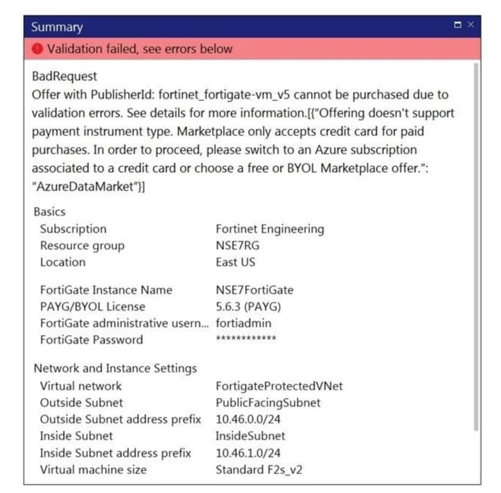
Refer to the exhibit. You are deploying a FortiGate-VM in Microsoft Azure using the PAYG/On-demand licensing model. After you configure the FortiGate-VM, the validation process fails, displaying the error shown in the exhibit.
