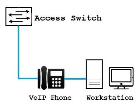
You have configured 802.1X single supplicant mode on the access switch. The VoIP phone does not support 802.1X authentication.
