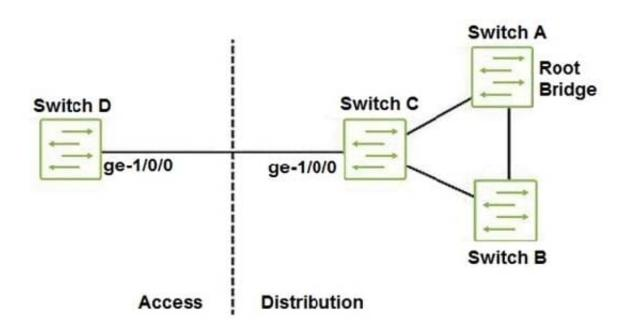
In the network shown in the exhibit, all switches are configured with the default STP root bridge priority, and Switch A has been selected as root. You recently added the older Switch D into the network as an access switch, and notice it has taken over as root.
