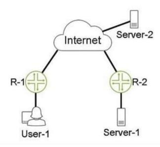
Referring to the exhibit, the GRE tunnel between R-1 and R-2 allows connectivity between User-1 and Server-1. When User-1 communicates with Server-2 with packets that are 1472 bytes in size, no packet fragmentation occurs. User-1 can communicate with Server-1 with packets that are up to 1448 bytes in size with no packet fragmentation. However, if the packet size is larger than 1448 bytes, packet fragmentation occurs.
