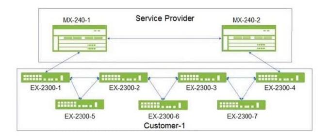
Customer-1 wants the Service Provider to allow STP to operate normally on all ports but only allow the MX Series devices to manage the Layer 2 topology.
