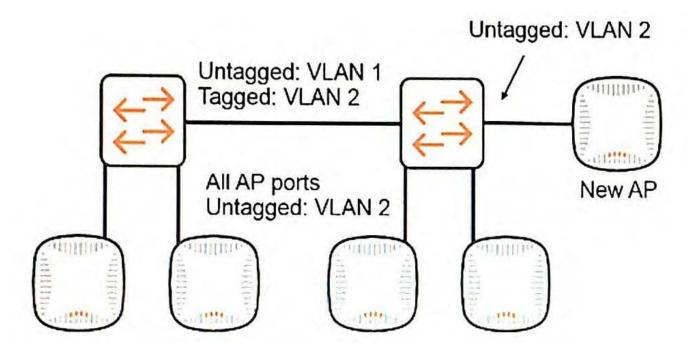
A company has an existing Aruba Instant cluster with several Instant APs (IAPs), as shown in the exhibit. The network administrator orders a new IAP and boots it for the first time by connecting it to the PoE switch port shown in the exhibit.
