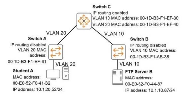
The Student A client needs to connect to FTP Server B. Student A sends the necessary ARP request and receives a reply. Which destination MAC address does the Student A client use in the FTP packet to FTP Server B?
