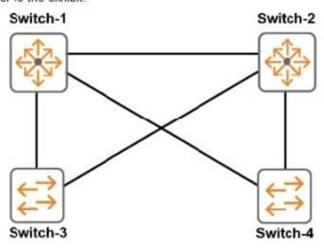
All switches are ArubaOS switches that currently have the default spanning tree priority. Switch-1 should be the root of the spanning tree If Switch-1 fails. Switch-2 should become root
