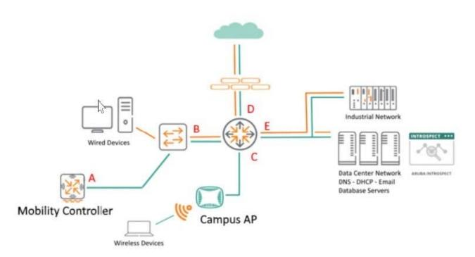
You are monitoring network traffic and considering DNS flow patterns. Where is a good location to place the Network Tap or Taps? (Location B will capture wired clients DNS requests while Location A will capture wireless client DNS.)
