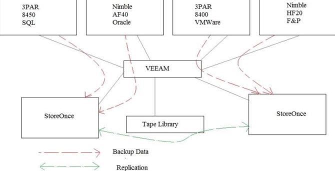
A customer has the environment shown. They currently perform application-consistent daily full backups via Veeam backup to an HPE StoreOnce device. These backups are then replicated to an alternate device using Catalyst copy.
