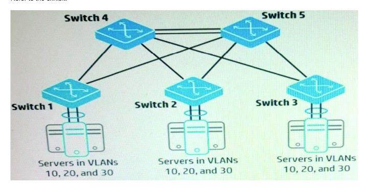
The switches shown in the exhibit form a TRILL region. What helps to load balance traffic across the .inks between these switches?
