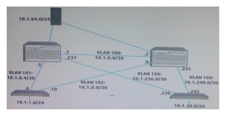
The exhibit shows the topology for a network with 30 access layer switches (only two are shown). Every switch-to-switch link is a Gigabit link. Every virtual local area network (VLAN) interface runs Open Shortest Path First (OSPF) and has
