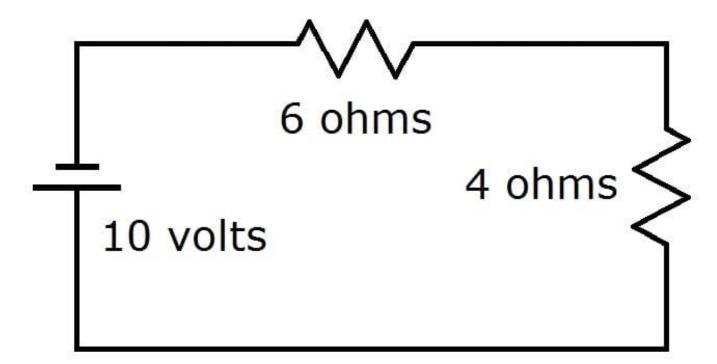
The current in the 4 ohm resistor is \_\_\_\_\_\_.
