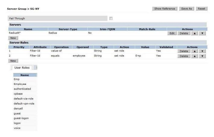
A user associated to an SSID with 802.1x using this server group. RadiusNY returned a standard radius attribute of filter-Id with a value of "employee".
