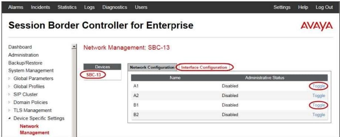
3. Click the Toggle link for both the A1 and the B1 interfaces. The Administrative Status for both A1 and B1 changes to Enabled
