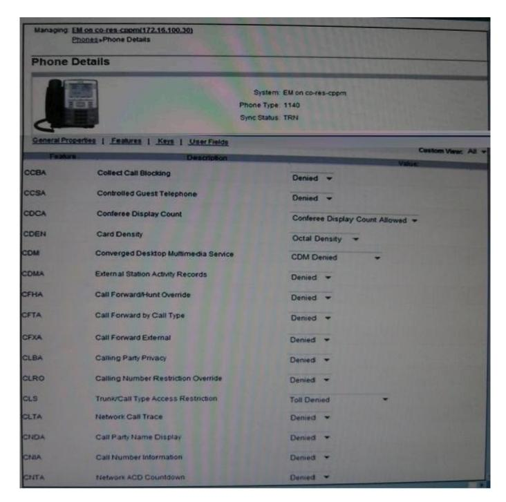
You manage a Communication Server 1000 RIs. 7 x system at a customer site. The customer reports that extension 2000 cannot make an unassisted long distance calls. With reference to the exhibit, which feature is restricting the user?
