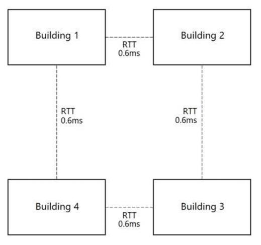
A university campus has a site topology illustrated in the exhibit. Adjacent connected buildings are connected with a single 40gb layer 3 network with a RTT of 0.6ms as depicted by each line. An architect wants to configure a fault
