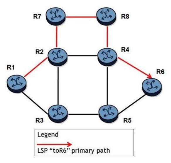
A fully loose LSP "toR6" is configured. All links have the same cost and all routers are Nokia 7750 SRs. The LSP currently traverses the path R1-R2-R7-R8-R4-R6 and the resignal timer is enabled. Which of the following about this LSP is FALSE?
