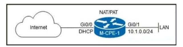
Refer to the exhibit. An engineer working for a service provider with an employee ID: 1234:56:789 notices that malicious traffic with a source IP in the RFC1918 range is arriving on the WAN connection to the internet and impacting customer resources on the LAN. Which ACL configuration must the engineer implement on M-CPE-1 to block the malicious traffic?
