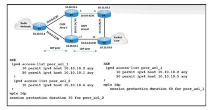
The radio network and packet core are using the route RX-RZ-RB to establish communication. The LDP session between 10.10.10.5 and 10.10.10.1 is experiencing link flapping at random intervals for 30-45 seconds each time. A network engineer must protect the LDP session and improve MPLS traffic convergence. Which action meets these requirements?
