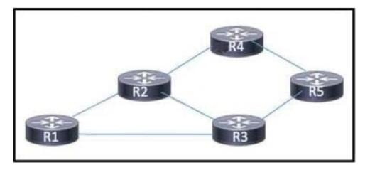
Refer to the exhibit. Routers R1 through R5 are being deployed within the core of a service provider running BGP. The core supports distribution of VPNv4 routes using MPLS. R3 currently has multiple paths to reach R4. A network engineer must implement BGP attributes so that R3 can reach R4 via R1. Which action must the engineer take to meet the requirement?
