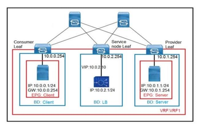
Refer to the exhibit. The client endpoint uses the load-balancer VIP as the destination address to send traffic to the server endpoint. If the load balancer does not do source NAT, which set of configurations must be applied on Cisco ACI to allow only the return traffic to be redirected to the service node?
