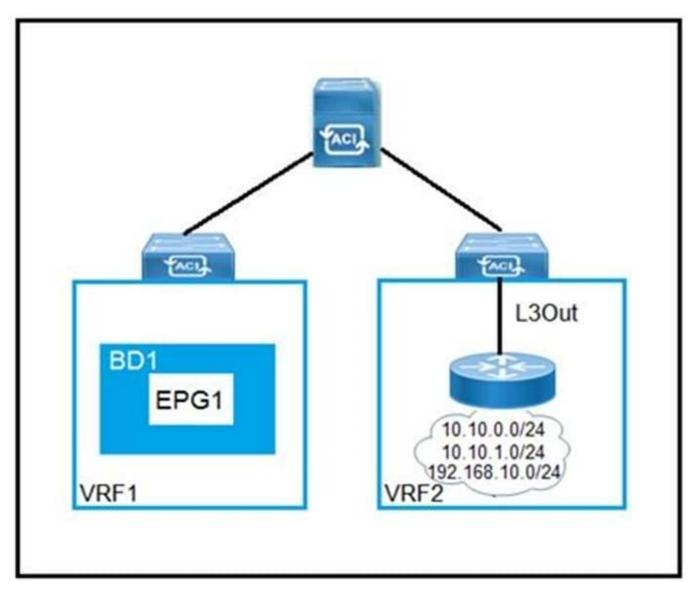
Refer to the exhibit. Drag and drop the subnets and flags from the left into the External Network Instance Profile policies on the right to create a setup that advertises only 10.10.0.0/24 and 10.10.1.0/24 prefixes in VRF1 and establishes connectivity between VRFs. Not all options are used.
