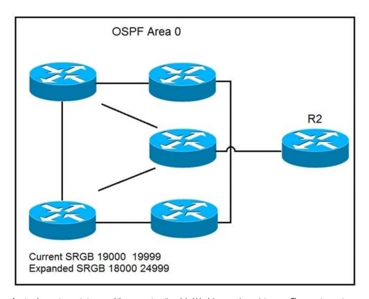
A network operator wants to expand the segment routing global block in upcoming maintenance. The operator must ensure that the changes to the segment routing global block have no adverse impacts on the prefix-sid associated with the loopback0 interface used within the OSPF domain.
