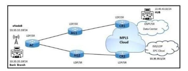
A service provider has LDP and segment routing running in the network. Mobility traffic is carried through LDP and enterprise traffic is carried through segment routing. Which configuration must be implemented to connect the bank branch with the HUB site on routers?
