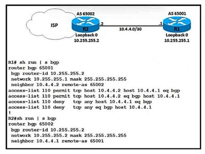
A network engineer notices that R1 and R2 cannot establish an eBGP peering. The following messages appear in the log:
