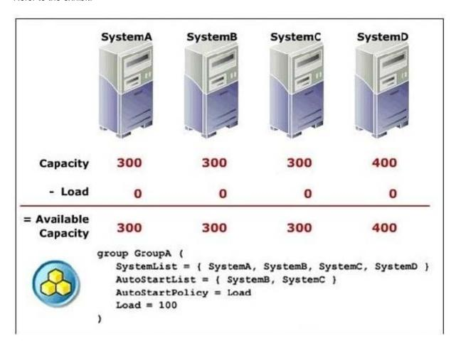
SystemC and SystemD are powered on. Subsequently, SystemA and SystemB are powered on. Where will GroupA start when the cluster comes online?
