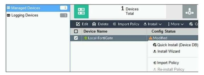
You are using the Quick Install option to install configuration changes on the managed FortiGate.
