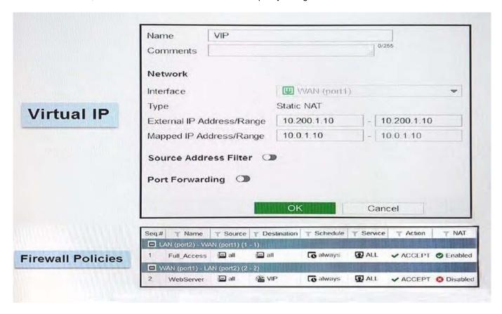
The WAN(port1) interface has the IP address 10.200.1.1/24. The LAN(port2) interface has the IP address 10.0.1.254/24. The top firewall policy has NAT enabled using outgoing interface address. The second firewall policy configured with a virtual IP (VIP) as the destination address. Which IP address will be used to source NAT the Internet traffic coming from a workstation with the IP address 10.0.1.10/24?
