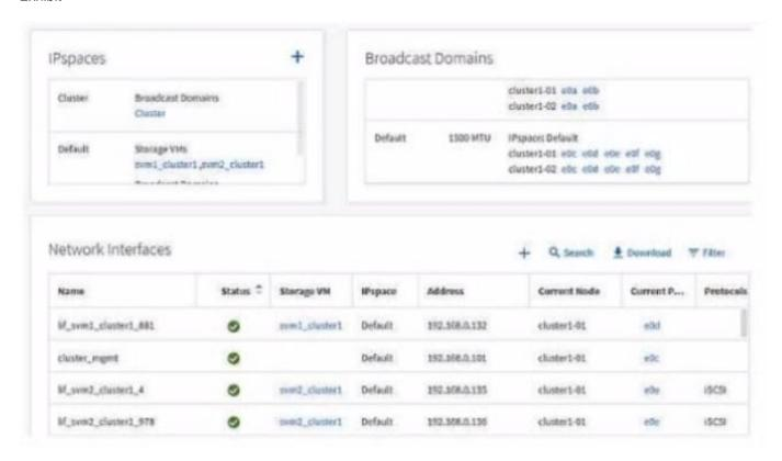
You have Installed a new ONTAP 9.8 cluster and want to move the e0e and e0c ports into a new broadcast domain. Referring to the exhibit, which action satisfies this requirement?
