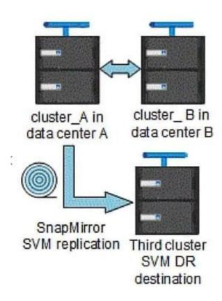
Using ONTAP 9.5, you are operating with data protection across three sites. The cluster\_A and cluster\_B systems require synchronous replication. The SVMs on cluster\_A also require asynchronous SVM-DR replication to a third site. All replication between all sites must also replicate the SVM configuration. Referring to the exhibit, which replication technology is supported between cluster\_A and cluster\_B?
