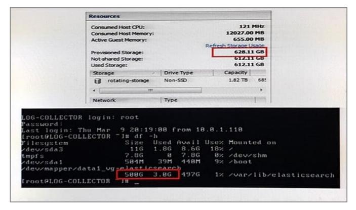
Referring to the exhibit, you have expanded the disk storage size in ESXi for your log collector from 500 GB to 600 GB. However, your log collector\\'s disk size has not changed.
