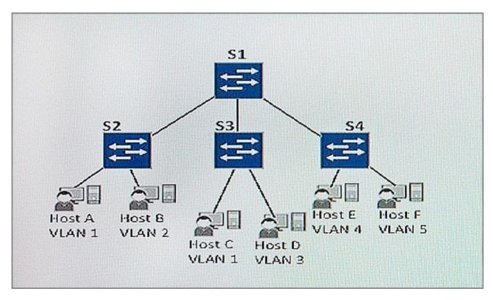
Referring to the exhibit, all interswitch links are configured as trunks supporting all VLANs. Host A sends a frame with an unknown destination MAC address to S2.
