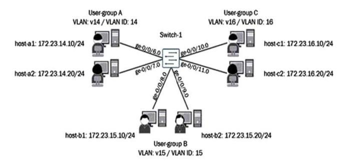
Referring to the exhibit, all users connected to the same VLAN can communicate with each other, but not with users on other VLANs in this network.
