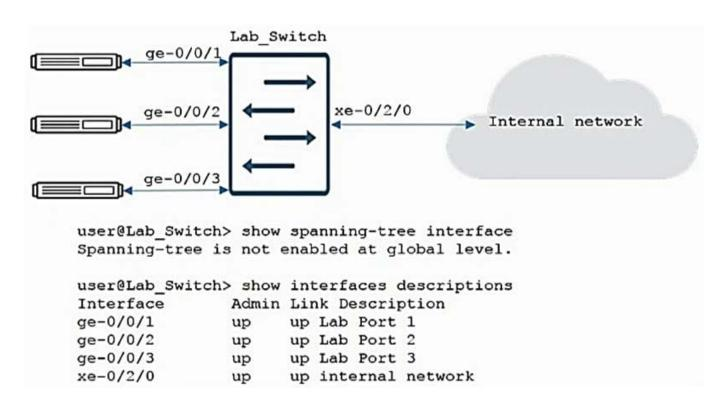
You want to prevent rogue BPDUs from lab devices reaching the internal through the Lab\_Switch device. Referring to the exhibit, what should be done to accomplish this task?
