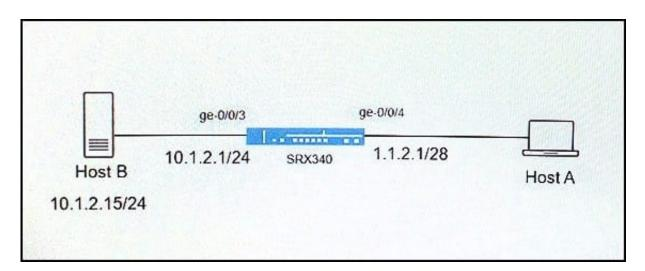
Host A is attempting to connect to Host B using the domain name, which is tied to a public IP address. All attempts to connect to Host B have failed. You have examined the configuration on your SRX340 and determined that a NAT policy is required.
