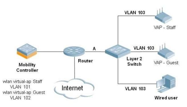
In the above diagram, the system shows two Aruba access points and a wired user.
