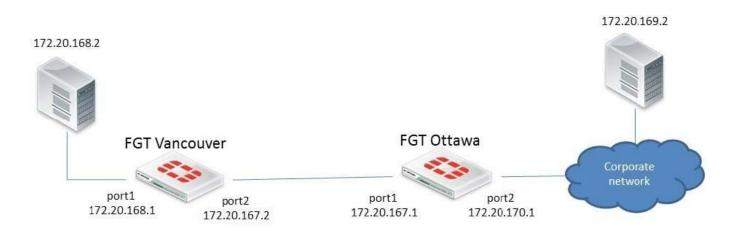
In this scenario, the Fortigate unit in Ottawa has the following routing table: S\* 0.0.0.0/0 [10/0] via 172.20.170.254, port2 C 172.20.167.0/24 is directly connected, port1 C 172.20.170.0/24 is directly connected, port2
