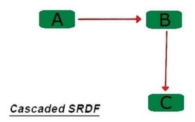
Cascaded SRDF has been deployed on VMAX3 has been deployed on VMAX3 arrays. The SRDF mode has been set to Asynchronous between Sites A and B.
