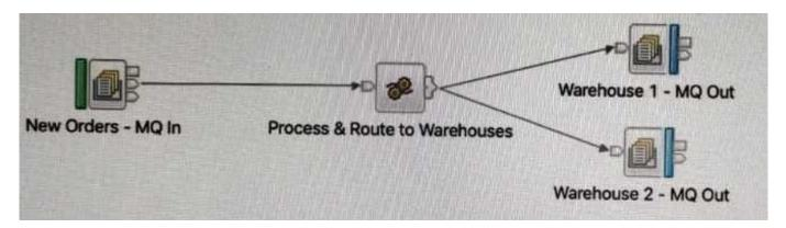
The compute node routes the message to two MQOutput nodes connected through terminals Out1 and Out using the following ESQL expressions. PROPAGATE TO TERMINAL \\'out1; RETURN TRUE;
