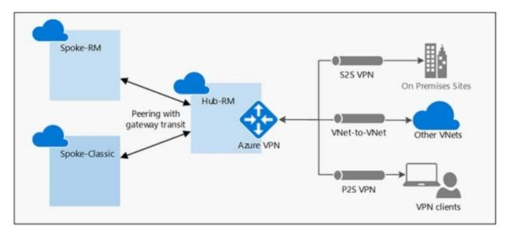
In the diagram, gateway transit allows the peered virtual networks to use the Azure VPN gateway in Hub-RM. Connectivity available on the VPN gateway, including S2S, P2S, and VNet-to-VNet connections,
