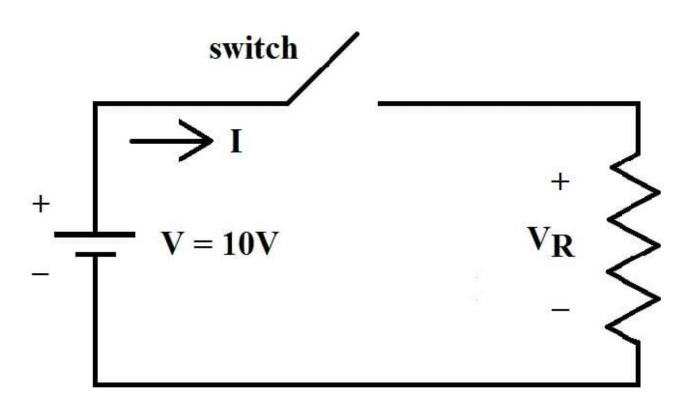
What is the voltage across the load R and the current through R when the switch is open in the following circuit?
