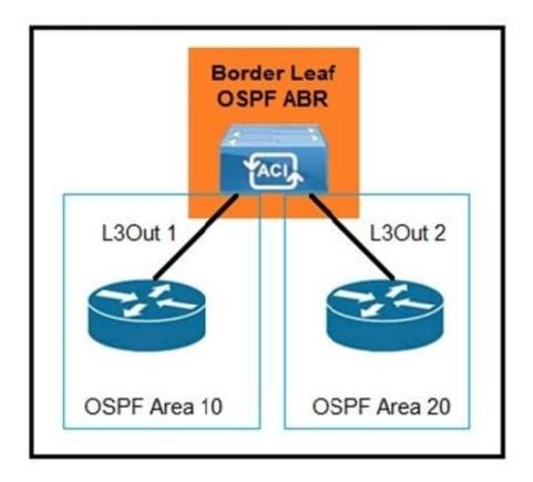
Refer to the exhibit. Which configuration must be implemented to allow intra-VRF transit routing between the two external routers?
