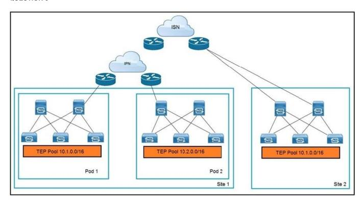
Refer to the exhibit. An engineer extends a Cisco ACI Multi-Pod setup to a Cisco ACI Multi-Site implementation. Which action allows the interconnection?
