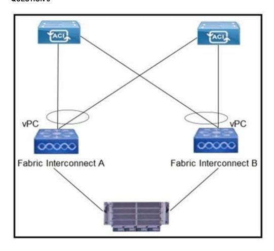
Refer to the exhibit. Which configuration mode must be selected for the VMM vSwitch Port Channel policy to avoid MAC flapping on the Cisco UCS Fls and Cisco ACI leaf switches?
