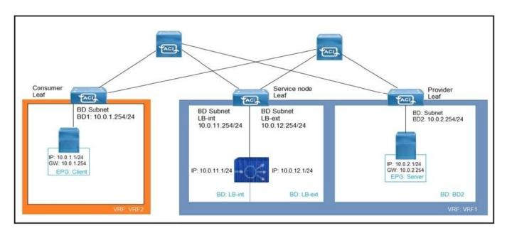
Refer to the exhibit. What must be configured to allow the PBR node (LB-int) to monitor the availability of the endpoint that is in the EPG server?
