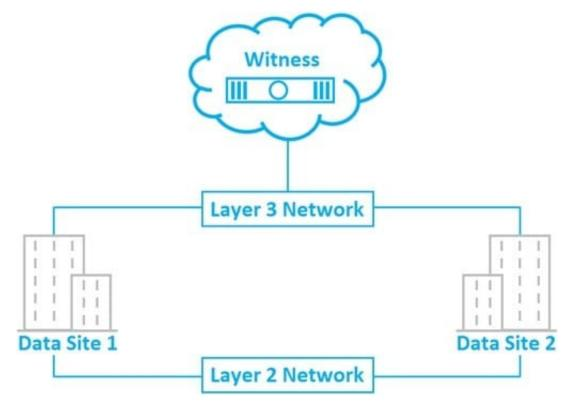
A vSAN Cluster stretched across Data Site 1 and Data Site 2 has a vSAN data network configured with an MTU of 9000. The witness node has been placed in a remote site across a WAN with an MTU of 1500. The vSAN health check, \\'vSAN: MTU check (ping with large packet size)\\', reports a failed ping.
