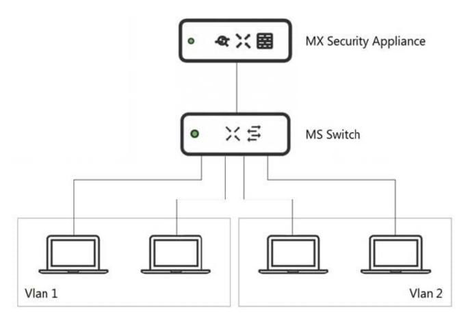
Refer to the exhibit. What is an advantage of implementing inter-VLAN routing on an MX Security Appliance rather than performing inter-VLAN routing on an MS Series Switch?
