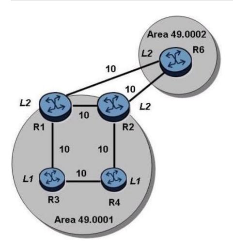
Examine the physical topology of the IS-IS network, the metrics of the links and the levels of the routers. All routers have a system address included in IS-IS.
