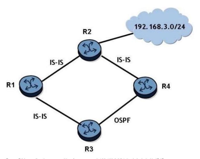
Router R2 has a directly connected interface to network 192.168.3.0/24 that is included in IS-IS.
