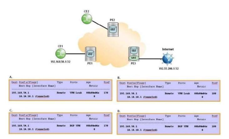
Internet access using route leaking between the VRF and the global routing table is configured in the network. Which of the following is the correct output of route 192.168.50.1 in the global routing table of PE3?
