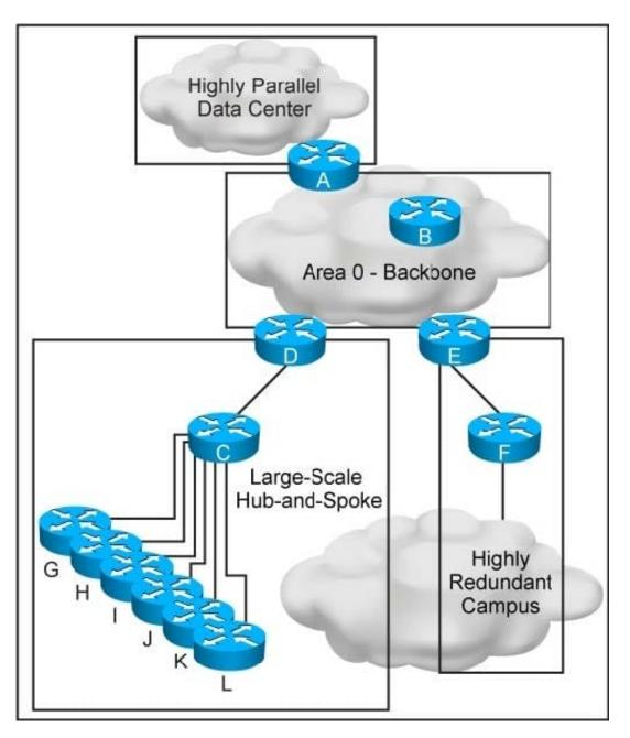
This OSPF network has just been deployed with four areas, but the hub-and-spoke area frequently flaps.
