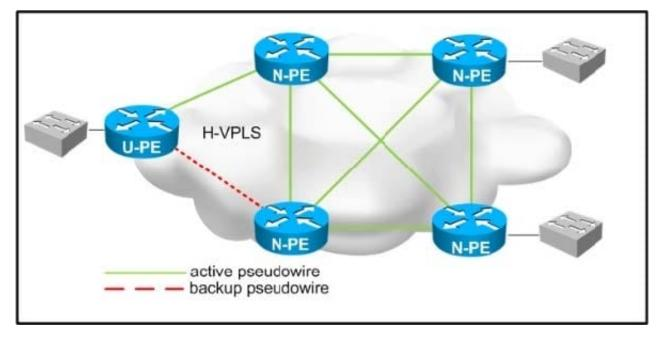
You are designing a loop-free hierarchical VPLS service. Which two design considerations should be implemented for the pseudowires between the N-PE and U-PE routers? (Choose two.)
