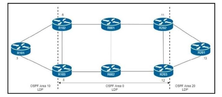
R101 is peering with R102 and R103, and R201 is peering with R202 and R203 using iBGP Labeled Unicast address families. The OSPF area 0 border routers are in a full iBGP Labeled Unicast mesh, and VPNv4 routes are exchanged directly between PE routers R101 and R201 through iBGP
