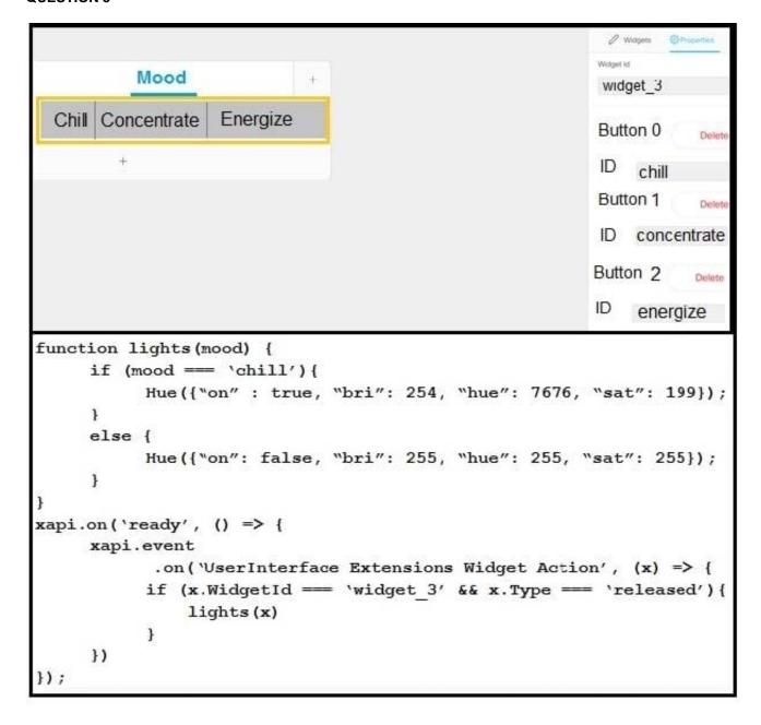
Refer to the exhibit. Certain lighting conditions are needed when hosting Webex meetings for a particular department in a company. A split button that integrates with the lighting controls is added to the Touch 10. However, when the user selects Chill, the lights turn off completely. Which code change resolves this issue?
