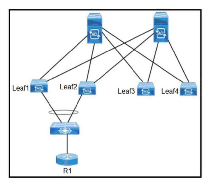
An engineer plans to upgrade the Cisco ACI fabric. Leaf1 and Leaf2 are deployed in a VPC. The fabric is peering with R1 using BGP protocol.
