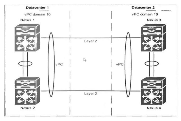
The administrator set up two pairs of Cisco Nexus switches. The administrator set dfferent vPC priorities on all four Nexus switches. As soon as the administrator activates the vPC between the two pairs the network faces different issues. The problems range from both Nexus pairs declare themselves as root bridge, as well as spanning-tree inconsistencies and traffic forwarding issues. Which action resolves these issues?
