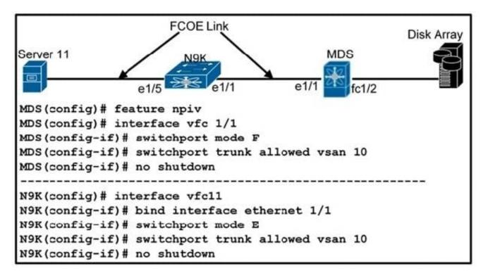
A network engineer is configuring the FCoE N\_Port virtualization storage area network. After the initial implementation, server 11 fails to connect to the disk array. Which action resolves the issue?
