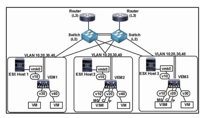
The VEMs fail to join a Cisco Nexus 1000V Series Switch. You determine that a system VLAN must be set on a systemuplink port profile. Which VLAN do you configure as a system VLAN?
