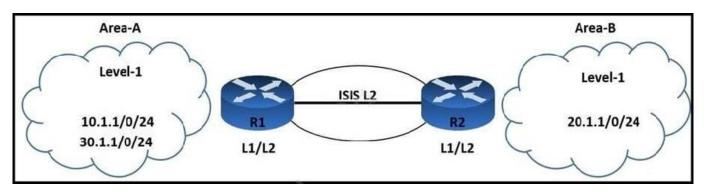
An engineer is troubleshooting IS-IS configuration between two areas. IS-IS Area-A network 30.1.1.0/24 is leaked into IS-IS Area-. R2 is failing to filter the route updates from network 10.1.1.0/24. Which configuration must the engineer apply to resolve the issue?
