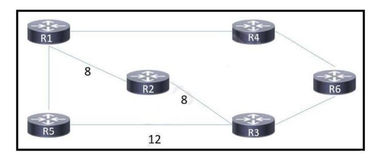
A network engineer configured routers R1 and R5 to run in IS-IS Level 1 mode and router R6 to run in IS-IS Level 2 mode. All other routers are running as Level 1 / Level 2 routers. An engineer expects traffic from R1 to R6 to pass via R2, but IS-IS routing has calculated the best path via R4. Which action corrects the problem?
