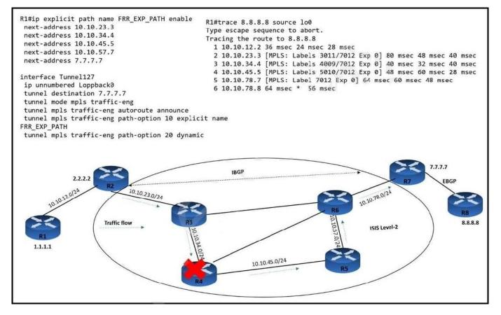
An MPLS core network has connectivity issues R4 has failed. It impacts traffic loss between R1 and R8. Customers report no access to their file servers, which delays their transformation work. Which quick action resolves the issue until R4
