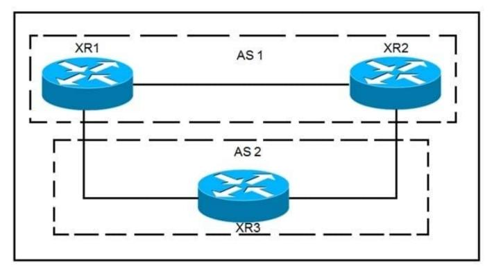
XR1 and XR2 are sending the prefix 10.11.11.0/24 to XR3. A configured policy on XR1 is incorrectly prepending AS path 11 11 12 12 onto this prefix. A network operator wants to add a policy onto XR3 that will not allow the falsely prepending prefix from being installed.
